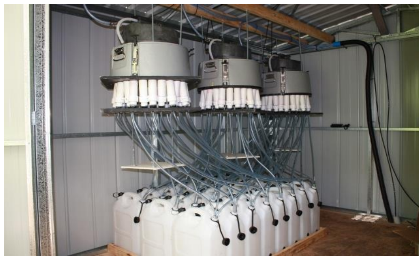
Figure 3: Automatic samplers setup at Fitzgibbon site with 24 x 20 L HDPE bottles.
