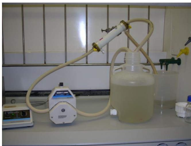
Figure 19: Stormwater sample concentration set up using Hemoflow HF80S dialysis filter.
