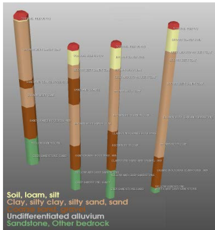
Figure 15: Examples of alluvial bore logs from the GVS software, showing (a) grouping into three categories, and (b) more detailed original geological logs.
