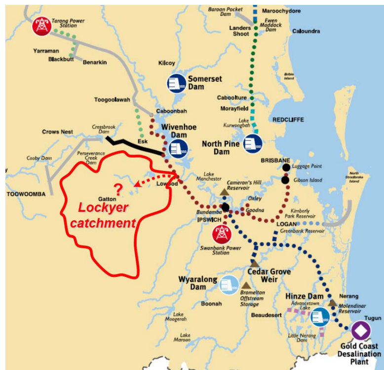
Figure 3: The Western Corridor Recycled Water (WCRW) scheme (red dotted line) in relation to the Lockyer Valley.
