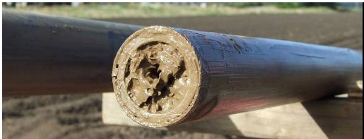
Photo 5: Liquefied 'super-saturated' layer of soil between 2.5–3 m in the Blenheim (B) soil profile.
