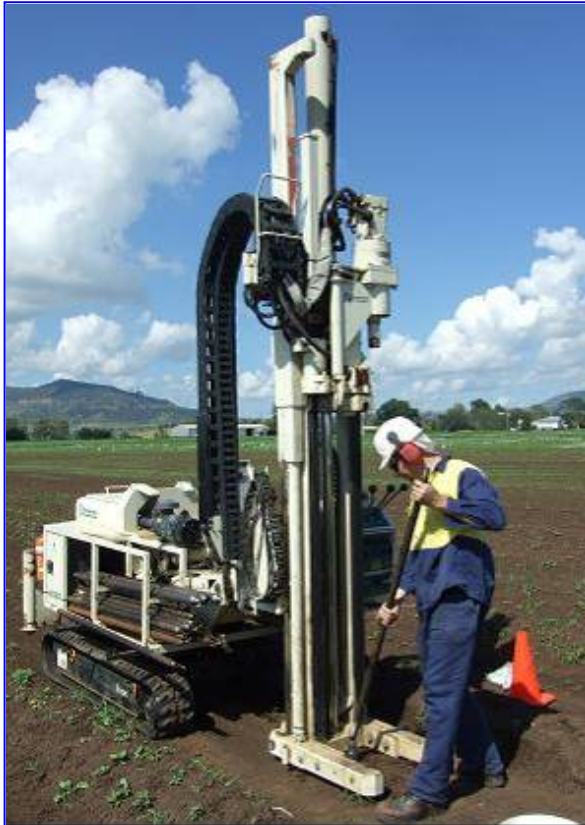
Photo 1: Geoprobe soil coring rig at the Tenthill site (operator Jeremy Manders).
