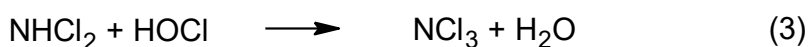
Figure 5: Monochloramine, dichloramine and trichloramine are formed from reaction between ammonia and hypochlorous acid.
