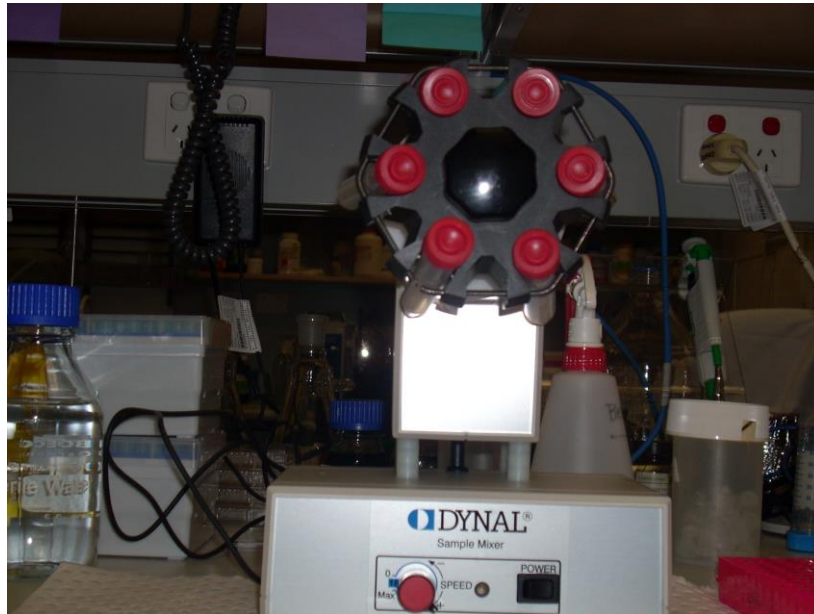
Figure 2. Mixing of tubes on a Dynal sample mixer to capture seeded virus in tap water samples.
