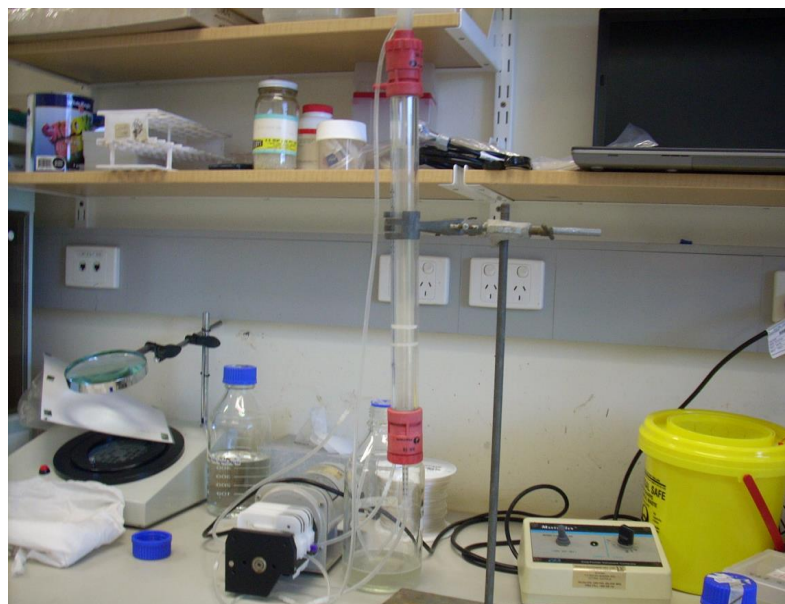
Figure 3. Modified chromatography column apparatus for virus concentration.
