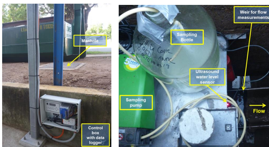
Figure 12. Flow proportional sampling set up. (Left view of the sampling site – right: view of the sampling system in the manhole).
