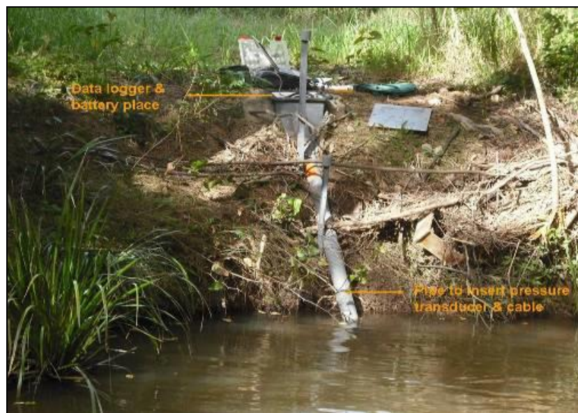
Figure 14: Pressure transducer and data logger placement at Upper Yuan Creek, Coomera (side view).
