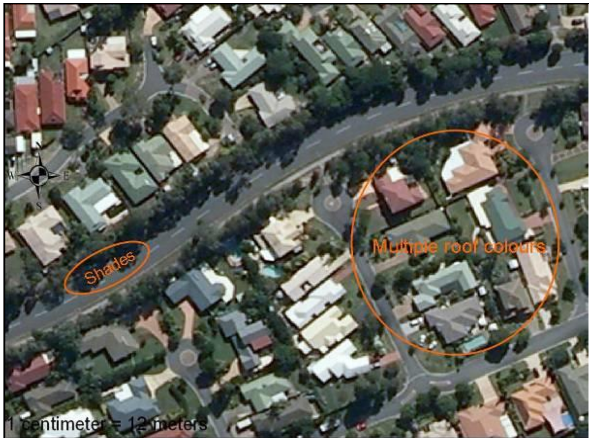
Figure 3: Two major constraints in image analysis processes, shading and multiple roof colours.
