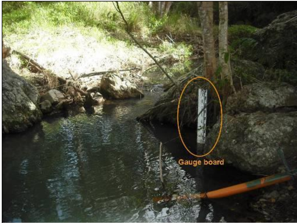
Figure 11: Gauge board installation at the Pimpama River, Kingsholme.
