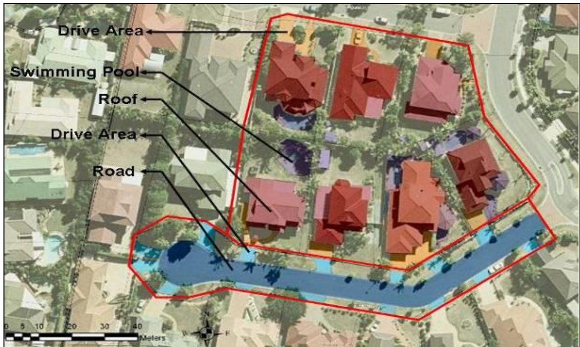
Figure 5: Manual digitisation of impervious area (roof, road, drive area and other paved surfaces such as swimming pool and tool shed) using the ArcGIS software.
