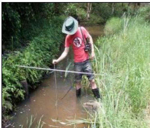
Figure 22: Low and medium flow gauging using a current meter (left) and high flow gauging using an Acoustic Doppler (right).
