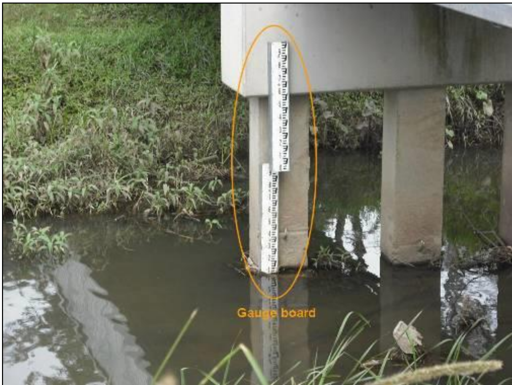
Figure 12: Gauge board installation at the Stable Swamp Creek, Rocklea.
