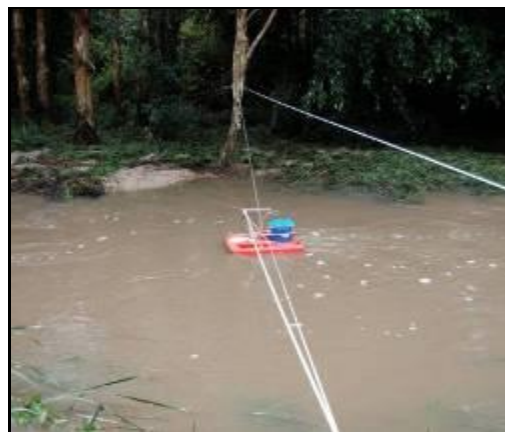
Figure 22: Low and medium flow gauging using a current meter (left) and high flow gauging using an Acoustic Doppler (right).
