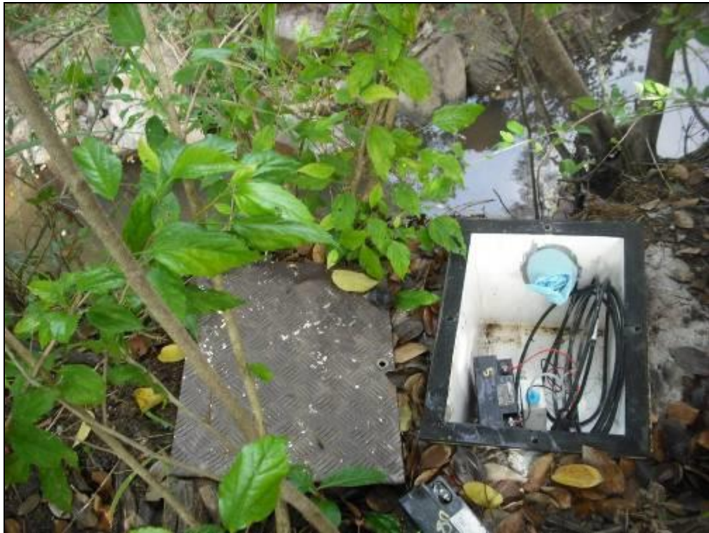
Figure 16: Replacement of battery of data logger / pressure transducer at Stable Swamp Creek, Sunnybank. The lid of the environmental enclosure is on the left of photo.
