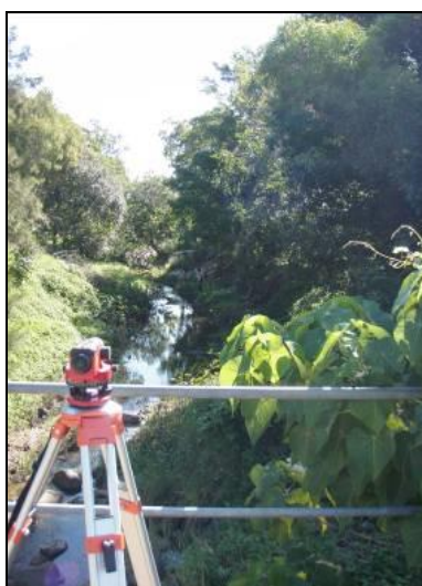
Figure 20: Surveying water surface slope at Stable Swamp Creek, Sunnybank using pegs installed during a prior high flow event.
