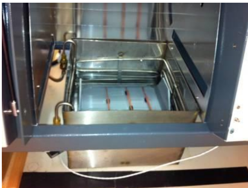
Figure 26. Overview of internal set-up of Solar Simulator, with cuvettes submerged and fixed in place within the temperature-controlled water bath.
