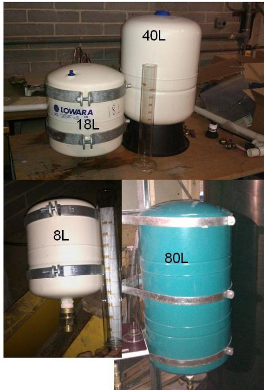
Figure 10: Pressure vessels examined: 8L, 18L, 40L and 80L nominal capacity.
