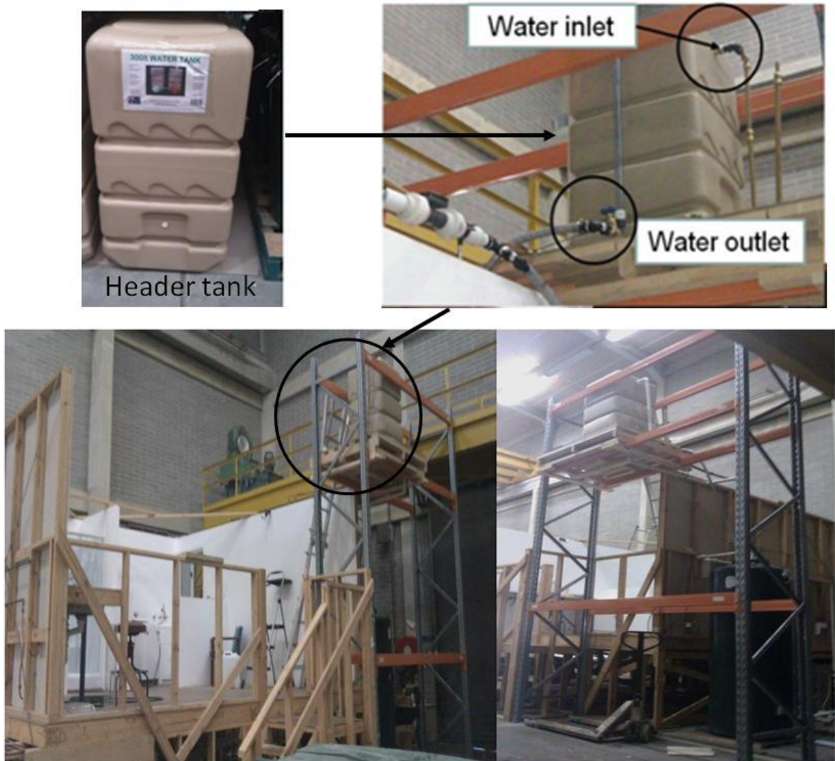
Figure 11: 300L header tank used in the analysis. It was located 2.7m above house floor level.
