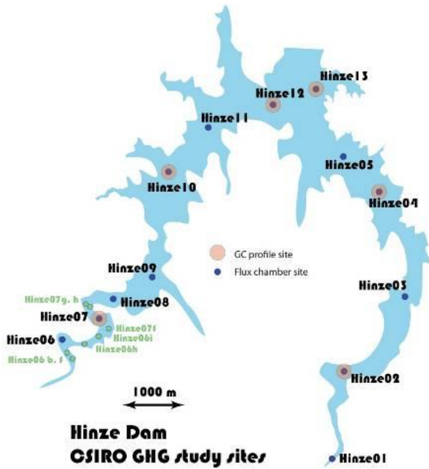
Figure 5: Hinze Dam methane flux measurement sites. Large red circles denote sites where dissolved methane concentration profiles were measured.
