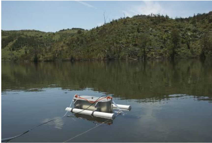
Figure 31: Floating chamber deployed in the field. Headspace gas is recirculated through the black and clear tubing. The ADV can be seen to the right of the chamber just below the surface.
