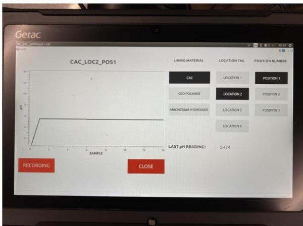
Fig 2. Hand-held tablet for displaying the real-time pH sensor measurements.
