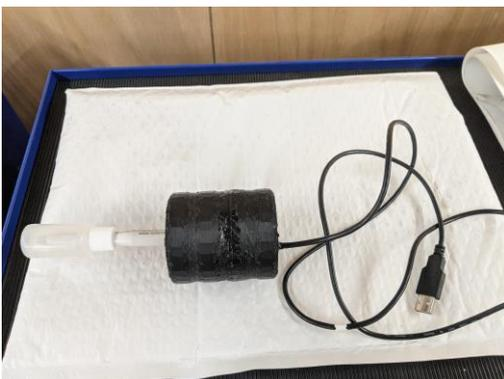
Fig 1. pH sensing system prototype.
