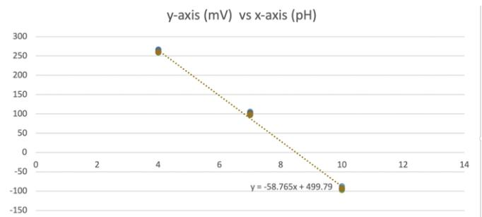
After calibration, multiple sensor measurements were taken in buffer solutions having pH levels 4, 7, and 10. The buffer solution pH levels were used as the benchmark. Table 1 presents the buffer solution pH levels versus the sensor measurements.
