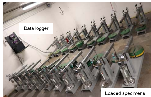
Figure 3. 20 creep rigs shown during creep testing in the basement of Civil Engineering Laboratory
