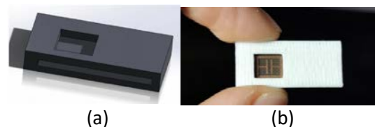
Figure 3: RFID sensor enclosure. (a) 3D CAD design. (b) Prototype.
