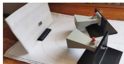
Figure 2: RFID sensor experimental setup with horn antenna.
