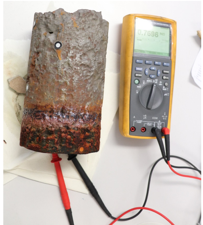
Figure 3. Image of Fluke handheld resistance multimeter and saturated CLCL pipe
