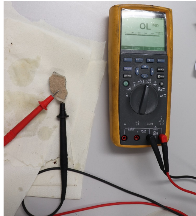
Figure 1. Image of Fluke handheld resistance multimeter and dry CML sample
