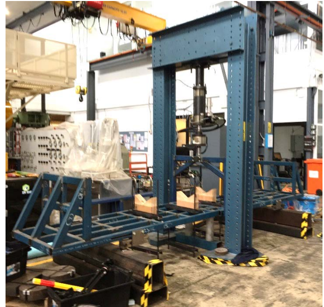
Figure 1: Pipe bending rig with clamps and supports
