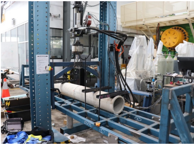
Figure 2: Test setup for trial 2, showing the use of metal clamps on an FRC pipe
