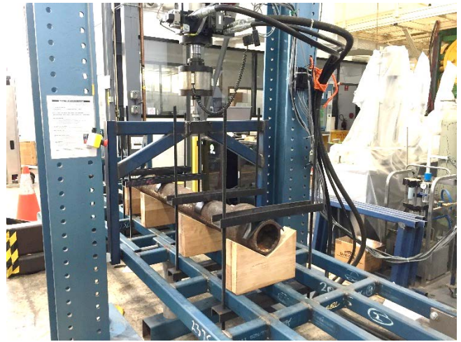
Figure 3: Test setup for trial 3 with wooden supports and metal clamps.
