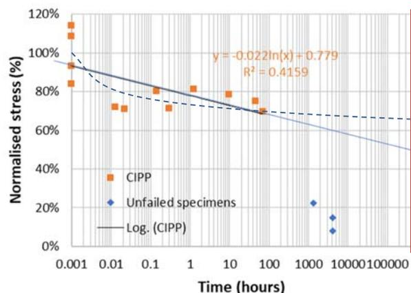
Figure 3. Normalised stress (%) (Creep rupture stress/maximum stress), vs. time (hours) in a log scale for CIPP liner tested. Curve was extrapolated for 50 years (red line). Blue dashed line proposed normalised stress vs. time curve.
