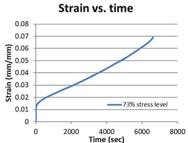
Figure 1. Strain vs. time curve of a tensile creep rupture test for spray liner subjected to a stress of 73% maximum tensile stress.
