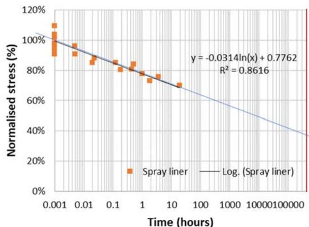
Figure 2. Normalised stress (%) (Creep rupture stress/maximum stress), vs. time (hours) in a log scale for spray liner tested. Curve was extrapolated for 50 years (red line).
