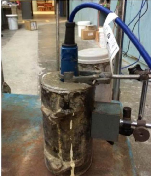
Fig. 22: pH Sensor monitoring in geopolymers sample. [21]
