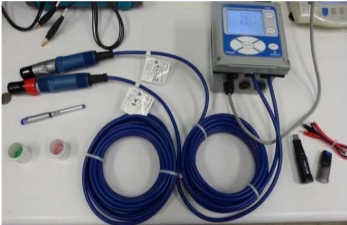
Fig. 21: pH Sensor System. [21]
