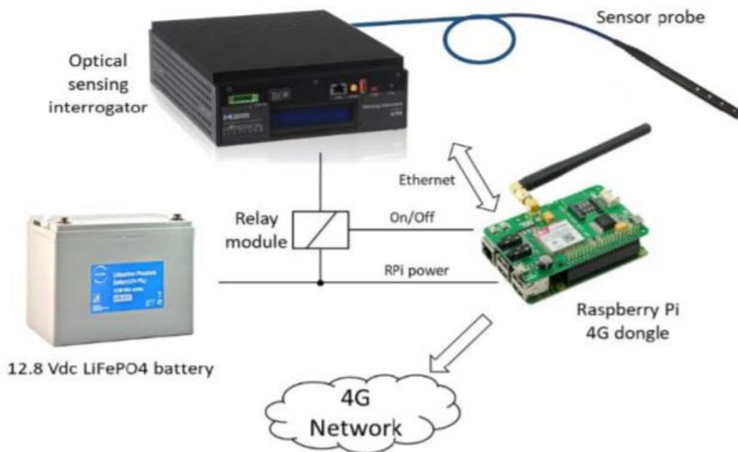
Fig. 20: Hardware setup for sensor monitoring and data collection. [18]
