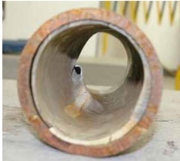
**Figure 1.** Uneven thickness in the spray liner (Ellison et al. 2010)
