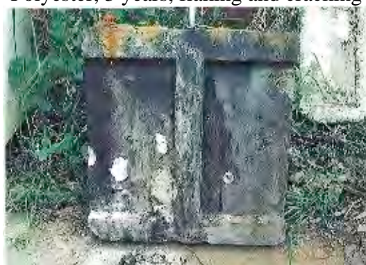
Polyester, 3 years, flaking and cracking
