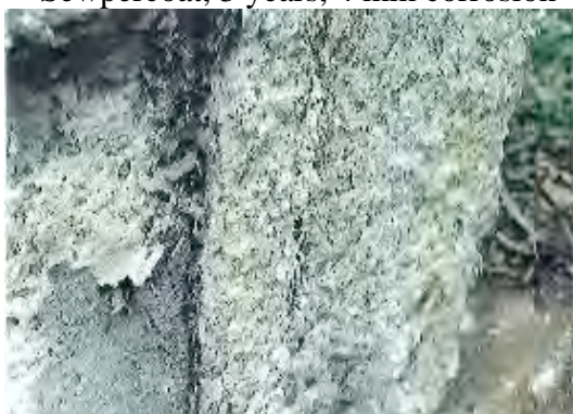
Sewpercoat, 3 years, 4 mm corrosion
