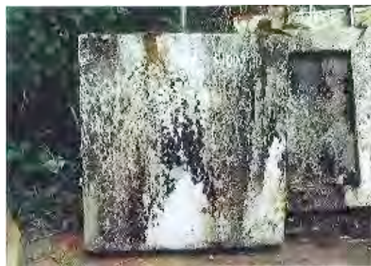
Polyester, 3 years, flaking and cracking
