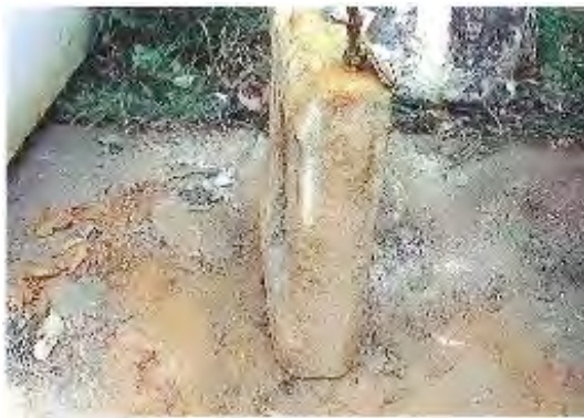
Sewpercoat, 3 years, 4 mm corrosion
