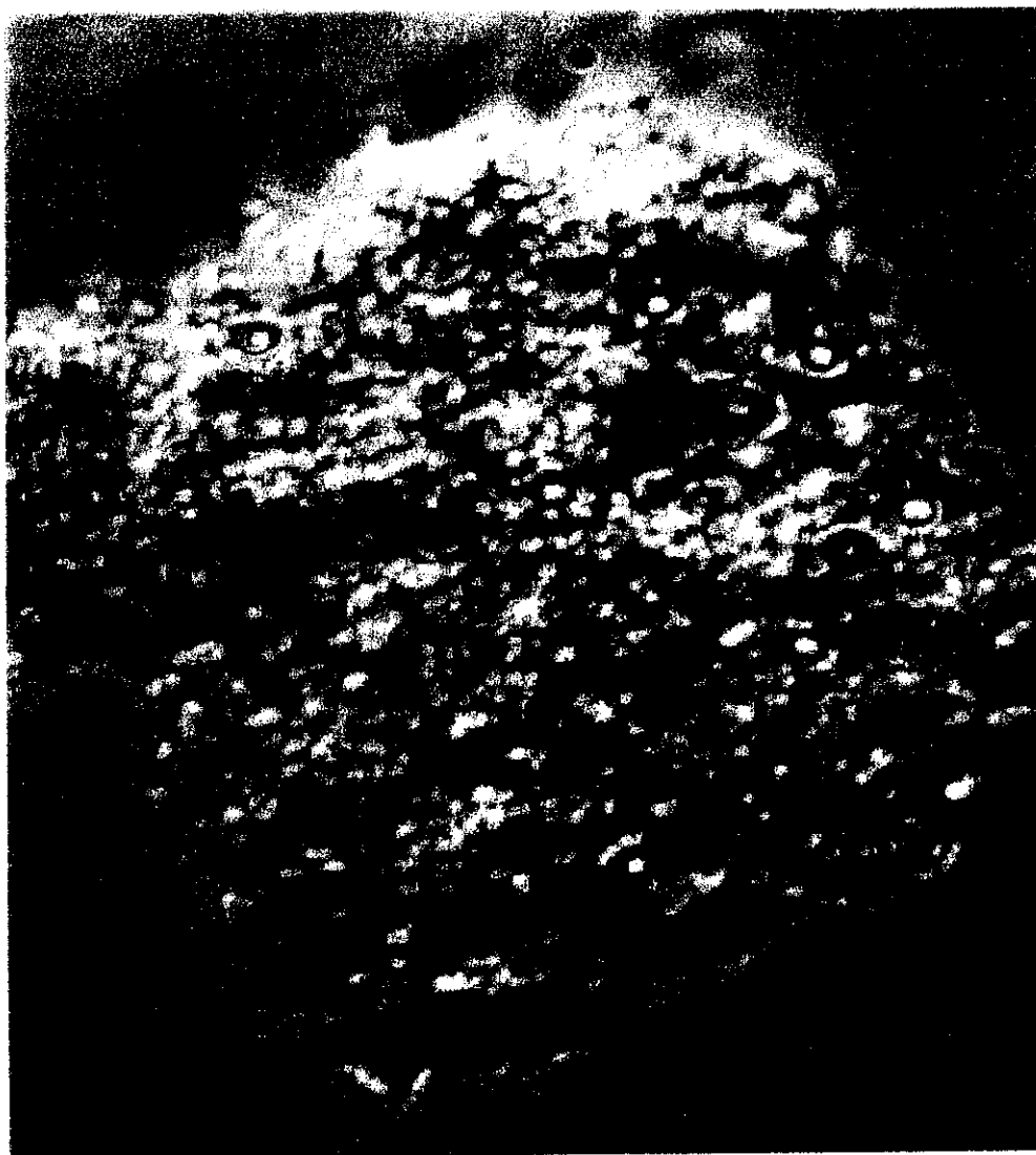
Figure 2.7b. Phase contrast photo of 5 \mu\text{m} latex particles trapped in a hydrous ferric oxide floc.
