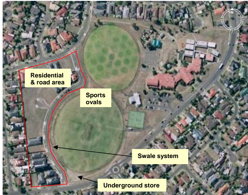
Figure 8: The Altona Green Stormwater Harvesting System (Source: modified from Google Earth)
