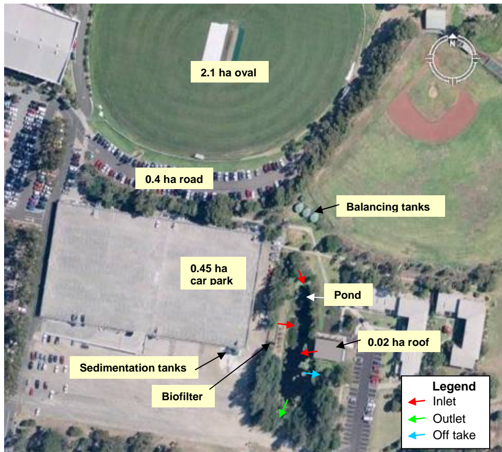
Figure 5: The Monash University Stormwater Harvesting System (Source: modified from Google Earth)
