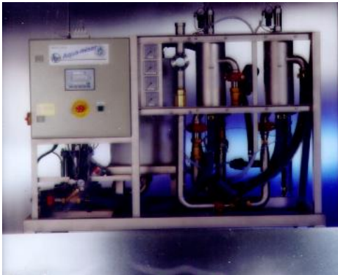
Figure 1. Picture of Aquamiser- Advanced Water Filtration Unit that filter water down to 25 micron and reuses in the pre-wash.
