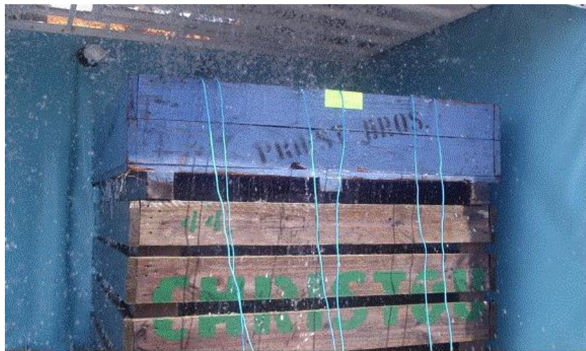
Figure 5.8. The box in which the instrumented pieces of broccoli were placed to measure their rate of cooling.
