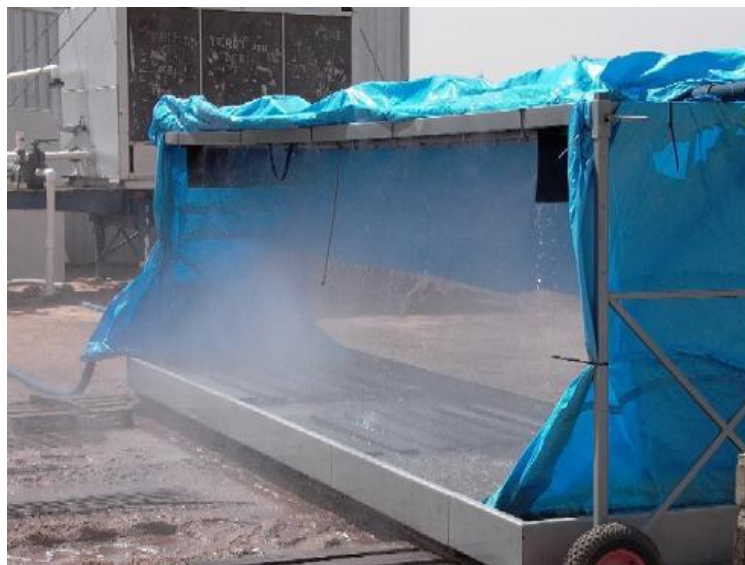
Figure 5.6. An alternative form of lightweight hydrocooler located on a property in southern Queensland. It consists essentially of a water collection tray in which pallets are placed on which the produce to be cooled is loaded. Water from the tray is recycled through the water chiller. Very little thermal insulation is provided.
