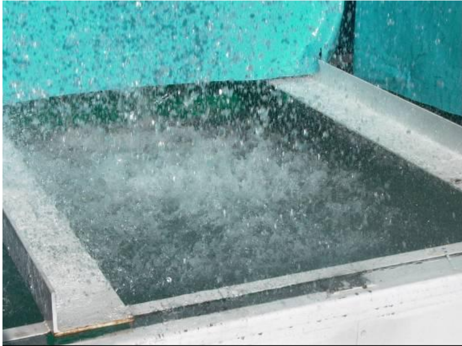
Figure 3.8. Wash water landing in the base of cooling bay 3.
