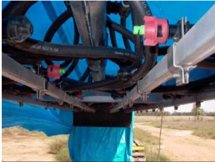
Figure 5.7. The water sprays in the Goondiwindi hydrocooler produce relatively fine droplets of water.
