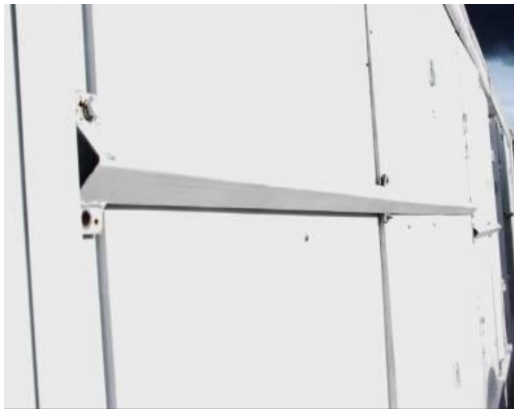
Figure 3.3. Each cooling bay is fitted with detachable doors that can be secured when the hydrocooler is being transported.
